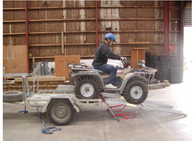
Correct procedure for unloading a quad bike from trailer. Rider wearing a helmet, all implements removed from the quad, trailer ramp in use, body positioned at the back of the seat, feet firmly on the foot pegs and a run-off area for the bike to ride out to
