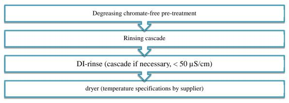
Beside the chromate-free corrosion protection process (product name) the used process variant is specified in the certificate of approval. As the approval test only includes the corrosion protection characteristics of the chromate-free pre-treatment product, the cleaning product will not be specified.
