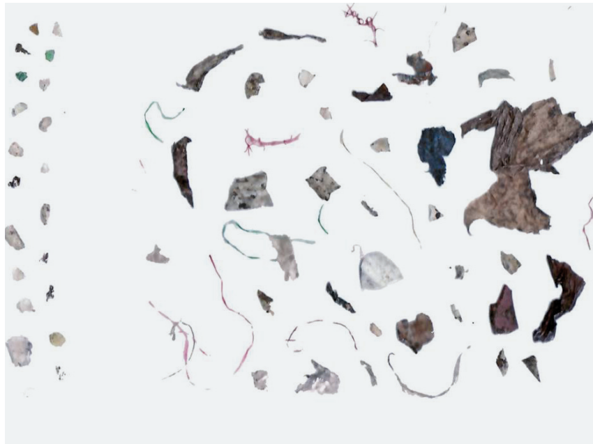
Impurities were sorted out of a 1 l digestate test sample.
