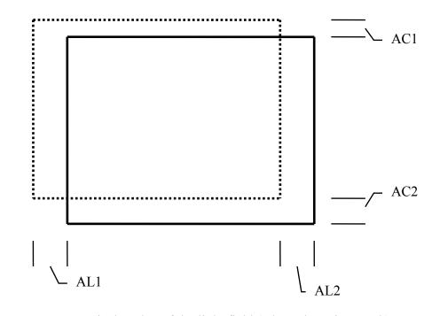
Where: ..... is the edge of the light field (where the coins touch) is the edge of the x-ray field
