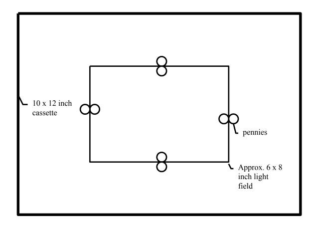
Figure 2. Setup for collimator accuracy test.
