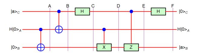
**Fig.37** The output after the step E;  $\frac{1}{\sqrt{2}}[|\beta_{00}\rangle_{CA} + |\beta_{01}\rangle_{CA}] \otimes |a\rangle$ . Immediately after Alice measures one of the Bell states  $(|\beta_{00}\rangle_{CA}, |\beta_{01}\rangle_{CA})$ , the state of Bob collapse into the state  $|a\rangle$ . The output after the step F;  $|0\rangle_{C} \otimes H |0\rangle_{A} \otimes |a\rangle_{B}$ .
