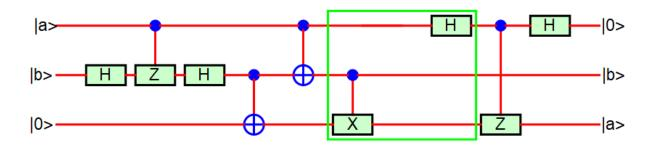
**Fig.31(e):** For the H and CX in the green box, with on change of the circuit, H can be shifted to the left, while CX can be shifted to the right within the box.
