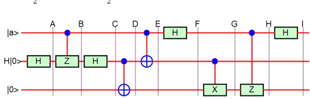
$$\frac{1}{2}|0\rangle \otimes |a\rangle \otimes X^{a}|0\rangle + \frac{1}{2}|0\rangle \otimes |a \oplus 1\rangle \otimes X^{a+1}|1\rangle$$
