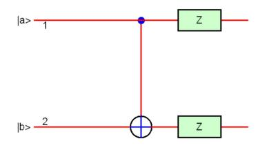
**Fig.12(b)** Quantum circuit equivalent to Fig.12(a).
