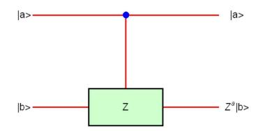
**Fig.8(a)** Controlled Z gate with control  $(|a\rangle)$  and target  $(|b\rangle, Z^a |b\rangle = (-1)^{ab} |b\rangle$ .
