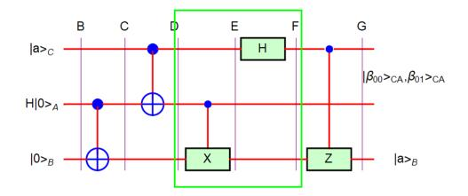
Fig.23(c) The change of location between H and X withing the green box. The element H shifts to the left, while the element X shifts to the right, without any effect on the output.
