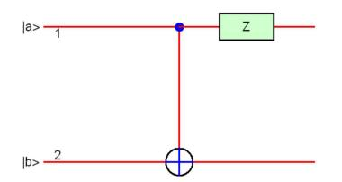
**Fig.14(b)** CNOT and Z-gate. Quantum circuit equivalent to the quantum circuit -4 of Fig.14(a). 1: control. 2: target. Input:  $|a\rangle \otimes |b\rangle$ . Output:  $(-1)^{a} |a\rangle \otimes |a \oplus b\rangle$ . Figs.14(a) and (b) are equivalent.
