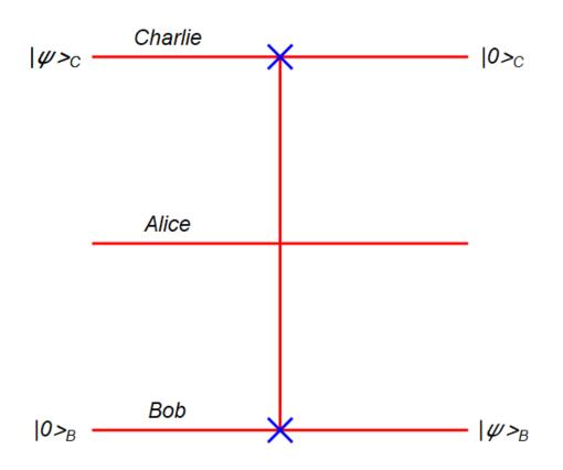
**Fig.24 (a)** SWAP circuit. Alice is not involved in this process. The result is independent of the choice of the state of Alice.
