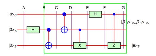
**Fig.23(b)** The change of the location of the input from the position A to B. The input at the position A is  $|a\rangle_C \otimes H|0\rangle_A \otimes |0\rangle_B$ .
