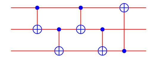
**Fig.24(b)** Equivalent circuit of SWAP, where the SWAP is replaced by CNOTs.
