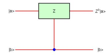
**Fig.8(b)** Controlled Z gate with control  $(|b\rangle)$  and target  $(|a\rangle)$ , which is equivalent to Fig.8(a)
