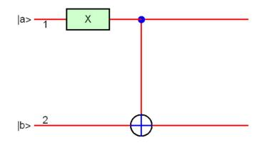
Fig.13(a) Quantum circuit-3.
