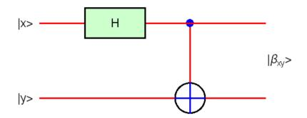
**Fig.9** Encode of Bell state  $|\beta_{xy}\rangle$ . Base transformation  $(|x\rangle \otimes |y\rangle \rightarrow |\beta_{xy}\rangle$  by H-CNOT gate.
