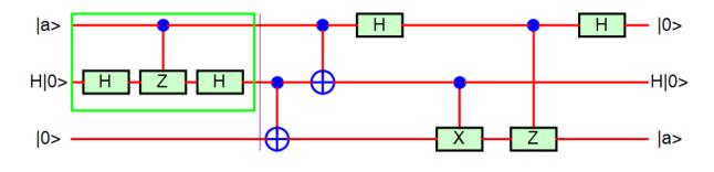
**Fig.35** No change occurs to the circuit upon the removal of the circuit element enclosed by the green box.
