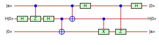
**Fig.34** SWAP. The output:  $|0\rangle_{c}$ ,  $H|0\rangle_{A}$ , and  $|a\rangle_{B}$ . The input:  $|a\rangle_{c}$ ,  $H|0\rangle_{A}$ , and  $|0\rangle_{B}$ .
