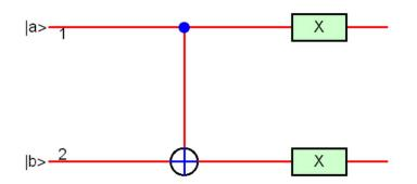
**Fig.13(b)** Quantum circuit equivalent to Fig.13(a).
