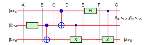
**Fig.22** Quantum teleportation circuit. The output after step-*G* is  $\frac{1}{\sqrt{2}}(|\beta_{00}\rangle_{CA} + |\beta_{01}\rangle_{CA}) \otimes |a\rangle_{B}$ . Immediately after Alice measures one of the Bell states  $(|\beta_{00}\rangle_{CA}, |\beta_{01}\rangle_{CA})$ , the state of the system collapses, leading the state of Bob into the state  $|a\rangle_{B}$ . In other words, the state  $|a\rangle_{C}$  of Charlie is transferred to Bob as the state  $|a\rangle_{B}$ .
