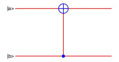
**Fig.16(b)** *CNOT* gate. Quantum circuit equivalent to Fig.16(a). Control gate ( $|b\rangle$ ) and target gate ( $|a\rangle$ ). The input: Input:  $|a\rangle \otimes |b\rangle$ . Output:  $|a \oplus b\rangle \otimes |b\rangle$ .
