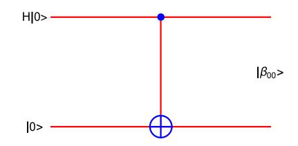
**Fig.6** Encode of the Bell state  $|\beta_{00}\rangle$  using CNOT gate with control  $(H|0\rangle)$  and target  $(|0\rangle)$ .
