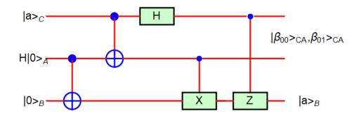
Fig.38 Equivalent circuit both for the quantum teleportation and the SWAP.
