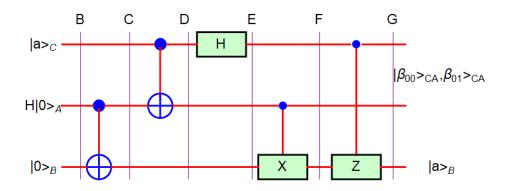
**Fig.23 (d)** Quantum circuit of quantum teleportation. The output at the line G is given by  $\frac{1}{\sqrt{2}} (|\beta_{00}\rangle_{CA} + |\beta_{01}\rangle_{CA}) \otimes |a\rangle_{B}$ . Immediately after Alice measures the Bell states (either  $|\beta_{00}\rangle_{CA}$  or  $|\beta_{01}\rangle_{CA}$ ), the state of Bob collapses to the state  $|a\rangle_{B}$ .
