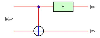
**Fig.10** Decode of Bell state  $|\beta_{xy}\rangle$ . Base transformation  $(|x\rangle \otimes |y\rangle \rightarrow |\beta_{xy}\rangle$  by H-CNOT gate.  $|\beta_{xy}\rangle = \frac{1}{\sqrt{2}}[|0\rangle \otimes |y\rangle + (-1)^{x}|1\rangle \otimes |\overline{y}\rangle$
