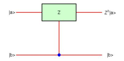
**Fig.15(b)** Controlled Z gate. Control gate  $(|b\rangle)$  and target gate  $(|a\rangle)$ .  $Z^{b}|a\rangle\otimes|b\rangle = (-1)^{ab}|a\rangle\otimes|b\rangle$ .Figs.15(a) and 15(b) are equivalent. CZ gate is non-local, independent of the choice of control and target.
