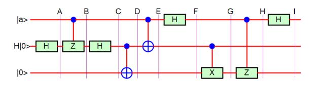
Fig.32 The equivalent quantum circuit for the SWAP.
