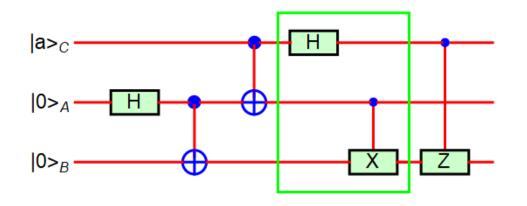
**Fig.20** The quantum circuit of quantum teleportation. Within the green box, the *H*-gate can be shifted to the right, while the *X*-gate can be shifted to the left. The output is not influenced by these shifts.
