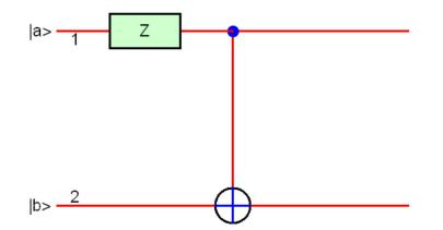
**Fig.14(a)** Z-gate and CNOT. Quantum circuit-4. 1: control. 2: target. Input:  $|a\rangle \otimes |b\rangle$ . Output:  $(-1)^a |a\rangle \otimes |a \oplus b\rangle$ .
