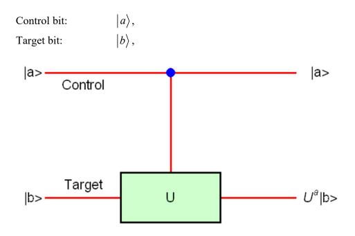
**Fig.2** Controlled U gate. Control  $(|a\rangle)$ . Target  $(|b\rangle)$ .
