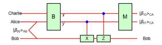
Fig.18Quantum teleportation circuit (Alice, Bob, and Charlie). The box B denotes<br/>the generation of the Bell state. The box M denotes the measurement
