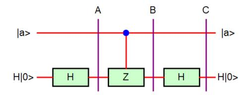
**Fig.36** Checking the possibility of removing *H*-*Z*-*H* gate.
