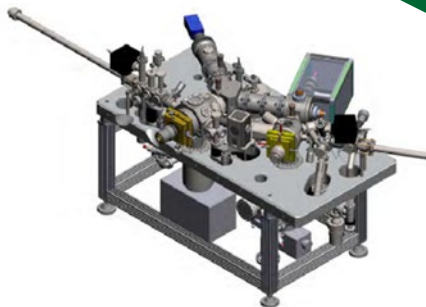
Quantum cryo-electron microscope with a spin polarized electron source to measure decoherence (LBNL)
