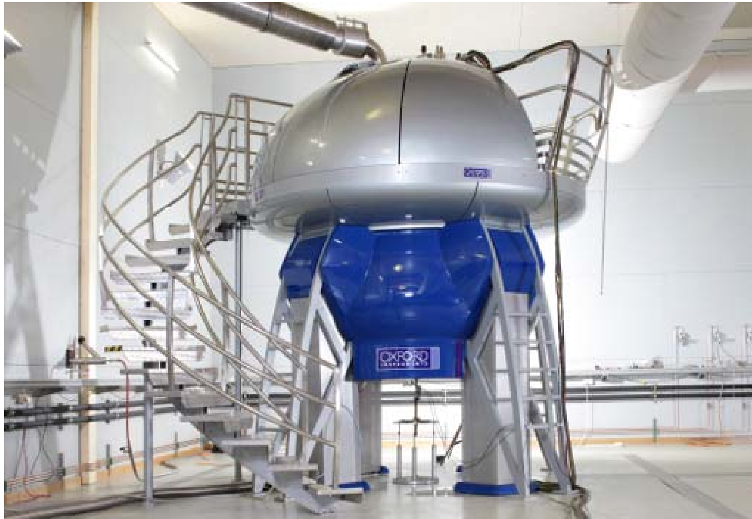
900 MHz NMR spectrometer for structural biology research in the Center for Biomolecular NMR jointly run by the Heinrich-Heine-Universität Düsseldorf und the Forschungszentrum Jülich.
