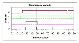
Figure 45. Discriminator output timing diagram for Example D.
