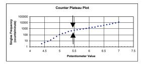
Figure 29. Example of counter plateau graph (log scale) used to determine optimal operating voltage of PMT.
