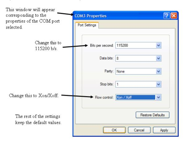
Figure 32. Where baud rate and flow control settings are modified for proper reading of the DAQ datastream with Hyperterminal.
