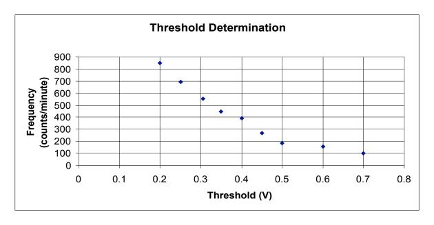
Figure 12. A graph of frequency vs. threshold for a counter used to determine threshold setting.
