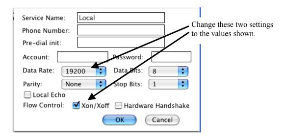
Figure 40. Where baud rate and flow control settings are modified for proper reading of the DAQ datastream with Zterm.
