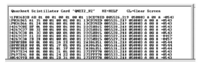
Figure 17. Sample screen of datastream from DAQ board when viewed with a terminal emulation program.
