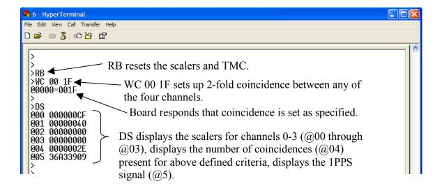
Figure 34. A sample terminal emulation window displaying how to set coincidence levels and how to read this coincidence data.
