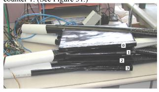
Figure 30. Shown here is a four-counter setup used in plateauing counters using the multiple counter method. Each counter is paired with another and coincidences are plotted over increasing voltages.
