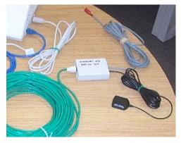
Figure 13. The GPS unit consists of a 100-ft. CAT-5 network cable (green cable), a GPS module (gray box), an antenna (black cable), and a temperature probe (gray cable, red end).
