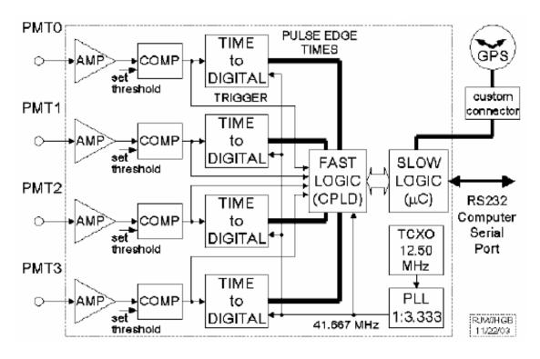
Figure 9. Block diagram of the QuarkNet DAQ v2.5 board..
