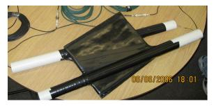
Figure 15. The latest version of the cosmic ray counter consists of scintillator, cookie (the flat paddle region), PVC pipe support (white cylinder, partially wrapped in black tape), and the PMT (black wrapped portion of the PVC pipe).
