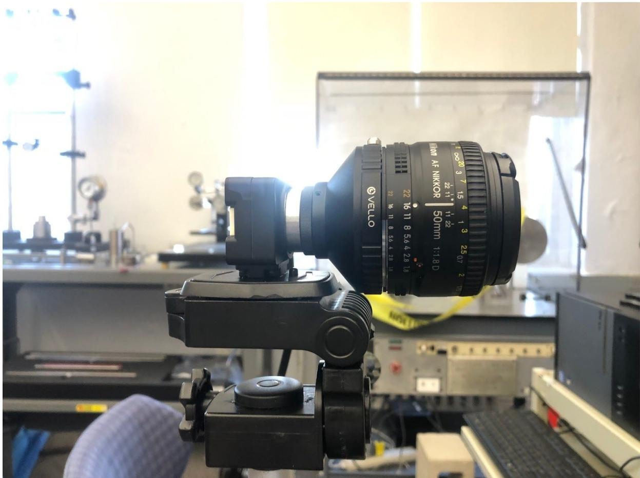
Figure (11): DIC Camera Setup with Lens and Lens Adapters
