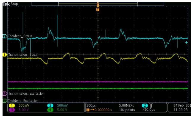
Figure 64: Example of spikes caused by a loose terminal
