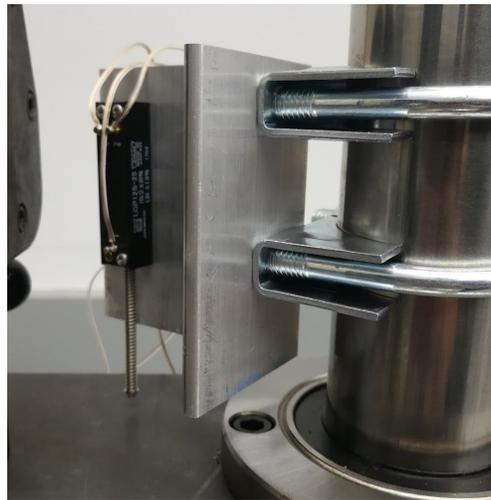
Figure (6): LCP12S Mounting Adapter
