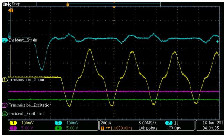
Figure 65: Example of overlapping waves on transmission bar.
