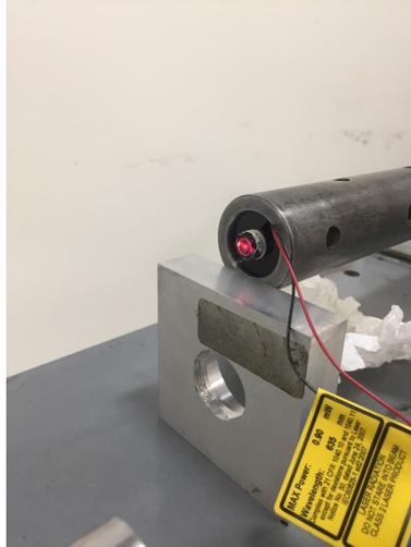
Figure 49: Laser Mounted Inside Gas Gun Barrel
