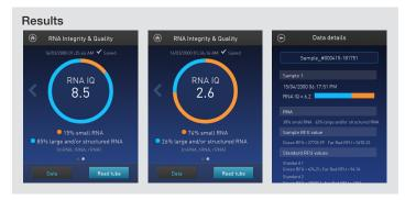
Figure 1. RNA IQ user interface on the Qubit 4 Fluorometer.
