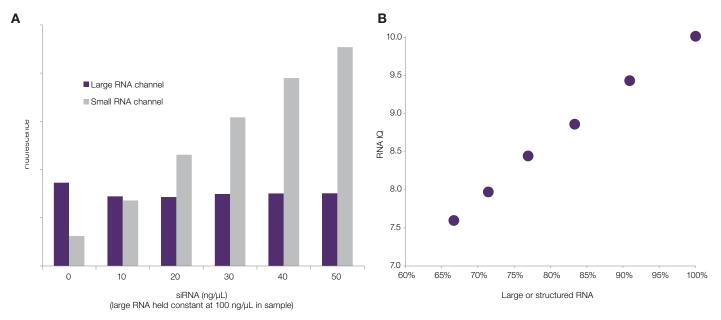
Figure 6. RNA IQ selectivity for large and small RNAs. (A) Fluorescence values obtained by the Qubit 4 Fluorometer are plotted for each type of RNA. (B) As expected, RNA IQ value increases with increasing percentage of large RNA.
