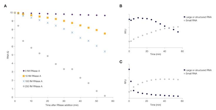
Figure 3. Real-time measurement of rRNA degradation by RNase A, using the RNA IQ assay. Results are plotted for (A) various concentrations of RNase A, (B) 10 fM RNase A, and (C) 100 fM RNase A.
