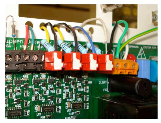
It is important to keep all exposed wire as short as possible, as exposed leads can short against each other or to ground, causing the panel to enter an alarm state.
