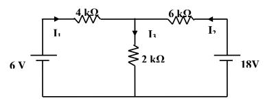
3. Determine the branch currents and voltage drops across each resistor.
