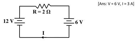
7. Find the total current and total resistance in the circuit given below.
