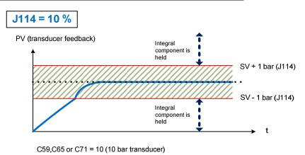
Figure 6.4: PID behaviour when function J114 is used.
