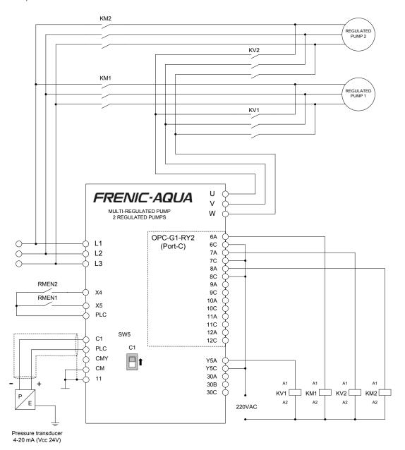
Figure 4.2: Schematics of multi-regulated pump control with 2 regulated pumps (Using OPC-G1-RY2)
