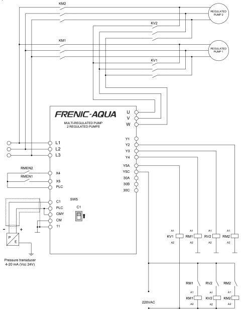
Figure 4.1: Schematics of multi-regulated pump control with 2 regulated pumps (Using additional relays)
