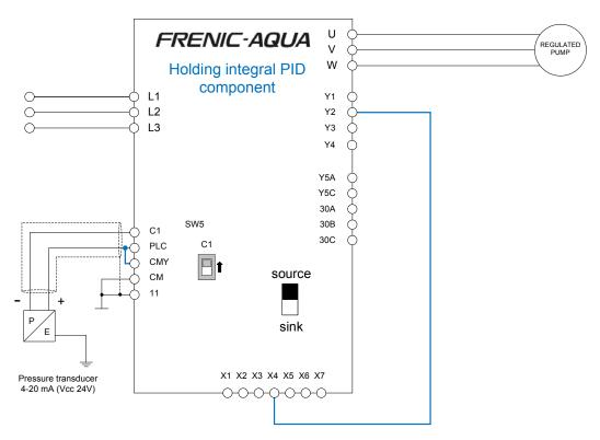
Figure 6.3: Pump control schematic for holding PID Integral component when pump is in sleep mode
