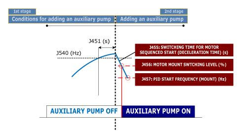
Figure 2.8: Auxiliary pump's connection
