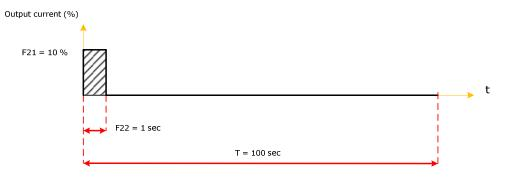
Figure 6.2: Output current when Dew Condensation prevention function is enabled
