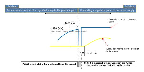
Figure 4.5: Connection of a regulated pump to the commercial power supply.
