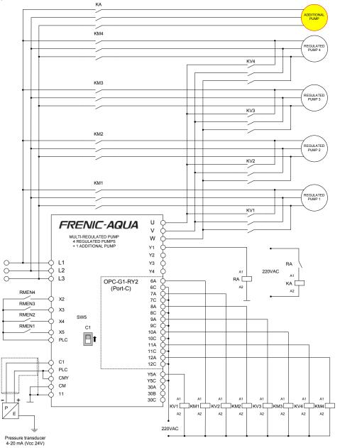
Figure 5.1: Schematic for multi-regulated pump control with 4 regulated pumps + 1 additional pump
