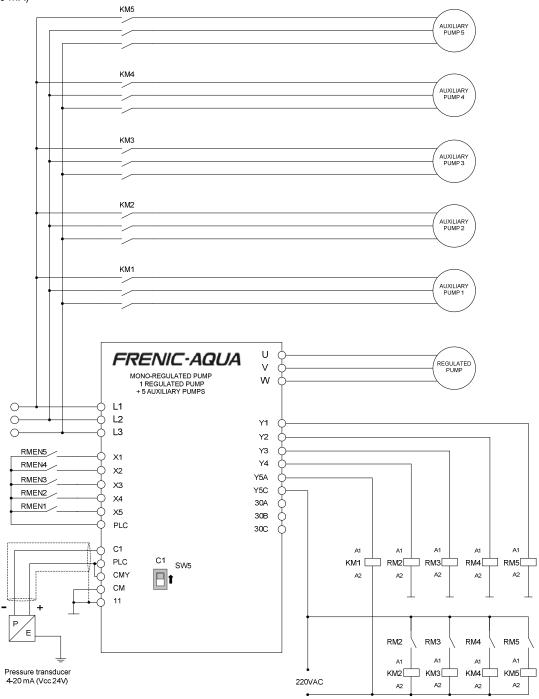
Figure 2.4: Schematic of a mono-regulated pump control with 1 regulated pump + 5 auxiliary pumps with external relays.
