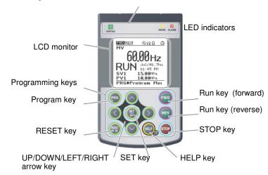
Figure 8.1: Names and Functions of Keypad Components
