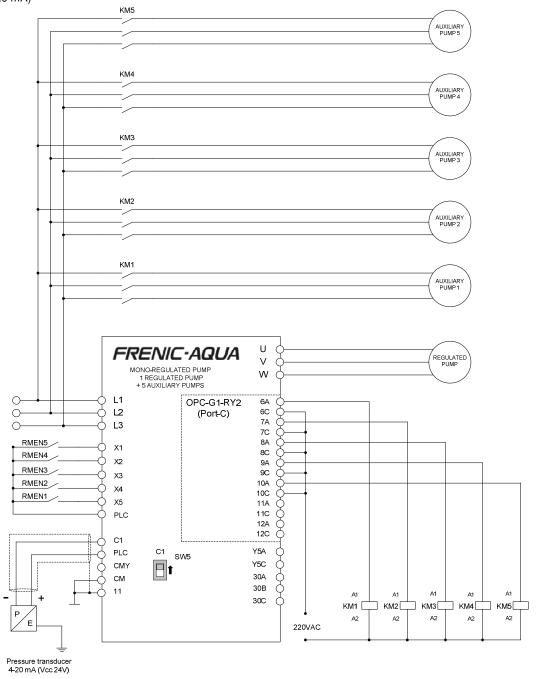
Figure 2.5: Schematic of a mono-regulated pump control with 1 regulated pump + 5 auxiliary pumps with option card.
