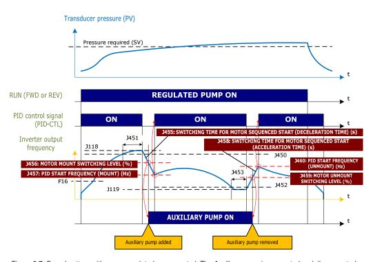
Figure 2.7: Speed pattern with mono-regulated pump control. The Auxiliary pump is connected and disconnected
