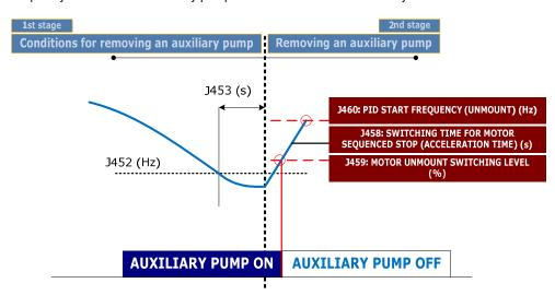
Figure 2.9: Disconnection of an auxiliary pump
