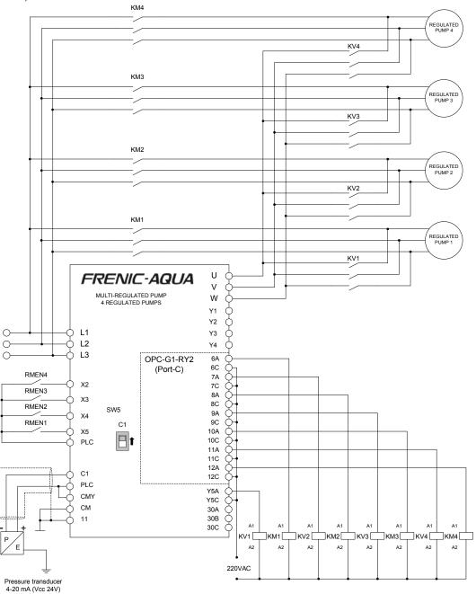
Figure 4.4: Schematics of multi-regulated pump control with 4 regulated pumps
