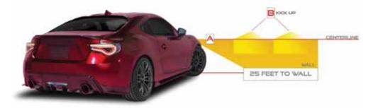
Look at the light pattern on the wall. Vertical aim: The top of the most intense part of the beam should be at or below the centerline of the headlamp horizontal tapeline. Horizontal aim: Most of the intense part of the beam should be to the right of the vertical centerline of the headlamp assembly.
