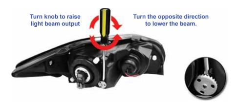
Next locate the tools that will be needed to adjust your headlamps. Note: Please do not ever use power tools on your adjusters this may cause severe damage to the internals of your lights.
