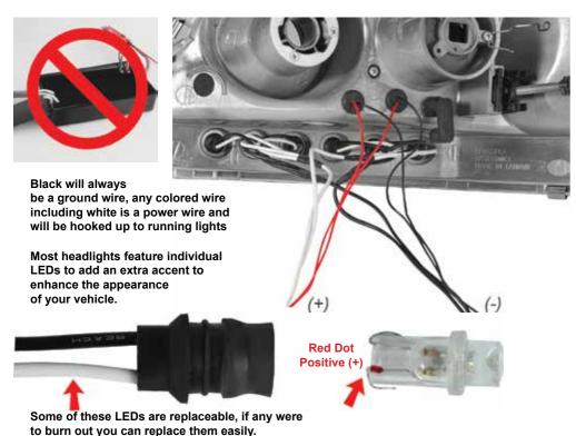
Spyder Auto headlights utilize a T10 LED bulb. Here are some directions on how to replace the bulbs:
