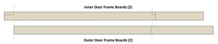
c. **Outer door frame boards:** Stand another 2X4 vertically on end against the outside of one of the door frame boards installed in 5.b. above so that it is resting on the inside edge of the baseboard and against the inside of the end bow. Position it such that its widest side is facing you. Using the end bow as a guide, make a mark on the 2X4 just under the bow.
