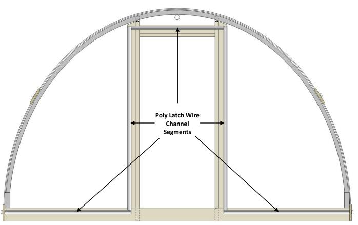
f. Hanging the door: Horizontally position the door over the doorway such that the edge that will have a hinge is in line with the point where the inner and outer door frame boards meet on that side of the doorway; confirm you have the same overlap on the opposite side (this should be 1½ inch or the width of the inner 2X4s.
