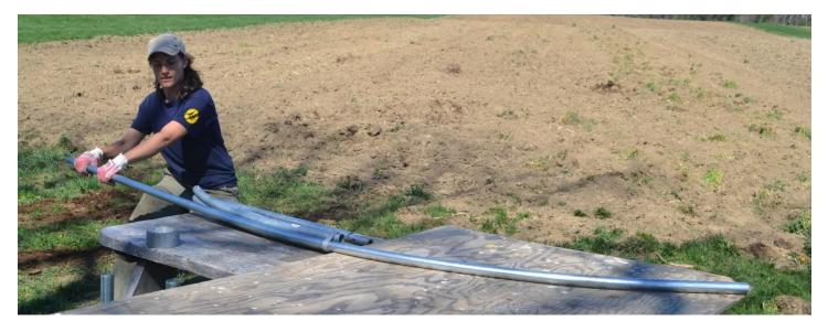
The Quick Hoops<sup>TM</sup> High Tunnel Bender may be mounted to any solid surface, such as a workbench, a picnic table, hay wagon, etc. It may be lag-screwed or thru-bolted into place.  ${}^{5}\!/_{16}$ " mounting holes are provided on the bender and the hardware to mount it are also included. By securing the bender in a fixed position, and pulling the tubing around the bender, the operator can maintain precise control of the tubing being bent.
