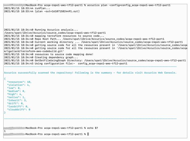
Accurics CLI returns "1" if high severity violations are detected, and "0" when there are no high severity violations.
