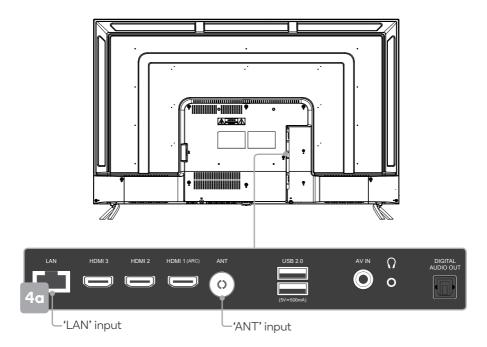
Following these options, the **Auto Tuning** screen will appear. Ensure you have an antenna cable connected to the 'ANT' input port at the back of the TV **(4a)**.
