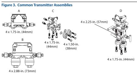
A. Transmitter with Coplanar Flange
