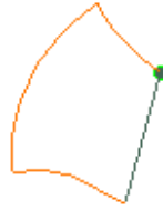
Open set of curves with its topological closing line (no curve is created as such, but as the edge of the trimmed surface, if any)
