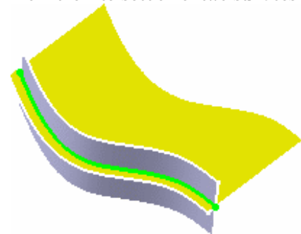
This example shows the curve resulting from the intersection of two surfaces
