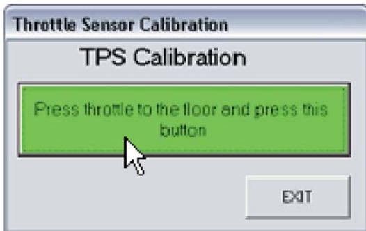
3) Wait a few seconds and the green calibration box will say "Calibration Complete." Your throttle position sensor is now calibrated.
