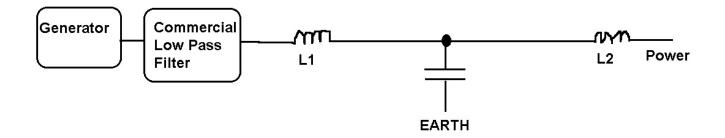
Model of Generator RFI Filtering
