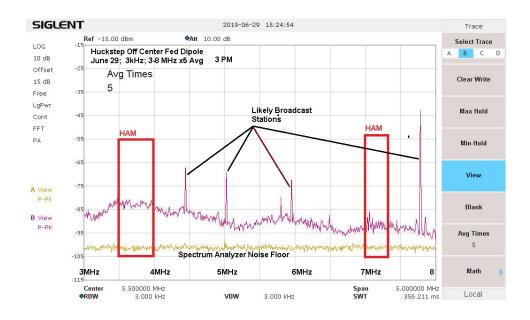
TAKE HOME: **Background HF 2.8 kHz noise is in the range of -85 to -95 dBm** in the lower HF ham bands, corresponding to S2 to S7 on the Icom 718. Generator noise ideally should be reduced below those levels.
