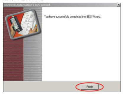
Now the EDS file has been loaded into RSLogix's database. Right-click the Ethernet menu item and select New Module.
