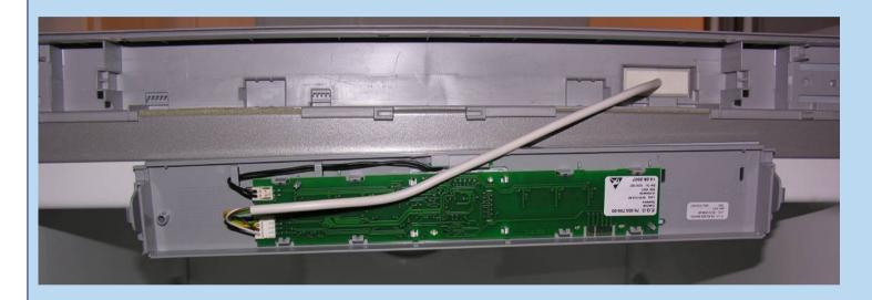
**Note:** Front panel is only replaceable as a complete unit, PCB is not
