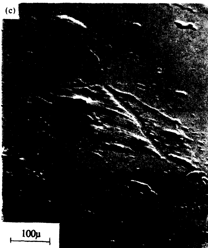
Figure 7. Optical (a) and SEM (b through d) micrographs of CEES-treated, PPZ-coated PET: (a) 30X; (b) 35X at a 66° tilt angle; (c) 170X at a 66° tilt angle; and (d) 400X at a 66° tilt angle.
