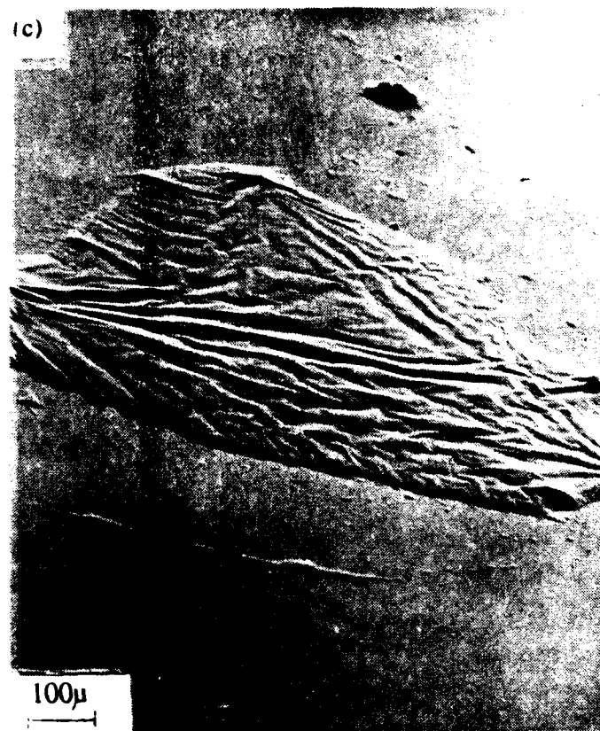
Figure 6. Optical (a) and SEM (b through d) micrographs of CEMS-treated, PPZ-coated PET. (a) 30X; (b) 35X at a 66^\circ tilt angle; (c) 100X at a 66^\circ tilt angle; and (d) 1000X at a 66^\circ tilt angle.
