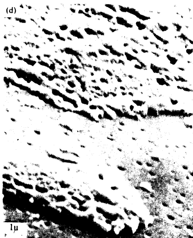
Figure 5. Optical (a) and SEM (b through d) micrographs of DIMP-treated, PPZ-coated PET: (a) 10X; (b) 170X at a 66^\circ tilt angle; (c) 1000X at a 66^\circ tilt angle, and (d) 7500X at a 66^\circ tilt angle
