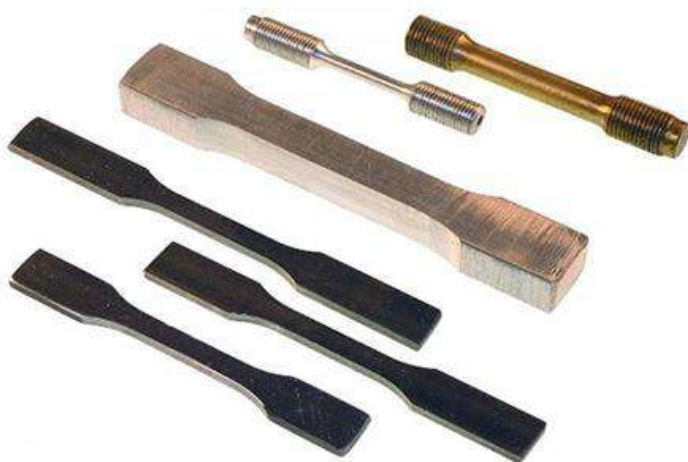
Fig (1) : Typical dog-bone specimens
