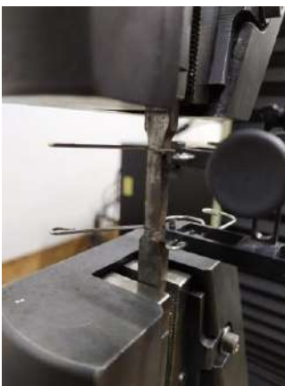
Fig (2) – Tensile testing machine at work
