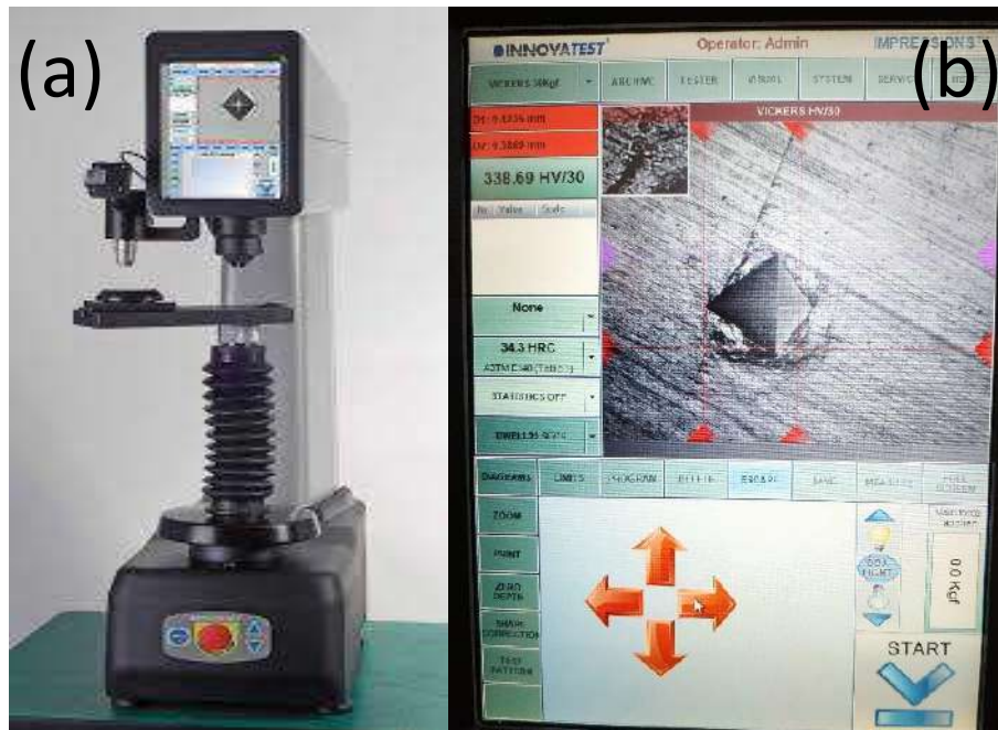
Fig.1: (a) Overall picture of the Vickers hardness tester and (b) picture of the operating monitor
