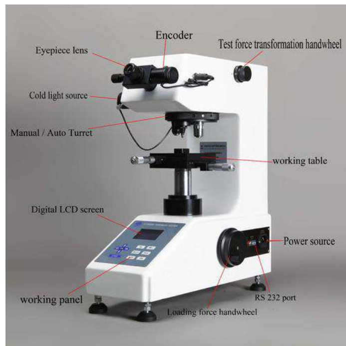
Fig. 3: A typical Vickers Microhardness Testing Machine
