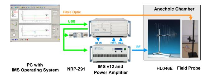
The block diagram shows the general setup of a test system according IEC / EN 61000-4-3. It covers radiated fields in the frequency range 80 MHz to 2 GHz. The field strength in 3 m test distance and over an area of  $1,5 \times 1,5$  m is 10 V/m. This configuration for 10 V/m is used by most customers.
