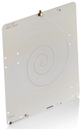
R&S®TS-F24WA1 broadband spiral antenna coupler 300 MHz to 6 GHz
