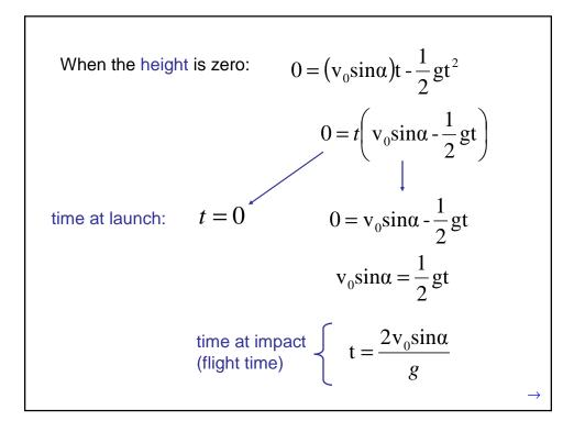
If we take the expression for flight time and substitute it into the equation for x, we can find the range.
