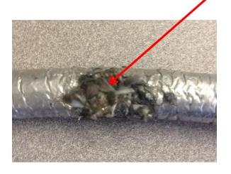
Visible fiberglass damage shown on Roush Fuel Line. If the heat sleeve is worn through to the point that the fiberglass is visible like shown, then it is recommended that it be replaced. As long as the line underneath shows no damage to the braid then a replacement sleeve can be installed over the line. Please contact ROUSH CLEANTECH at Phone Number: 800.59.ROUSH or e-mail ROUSHcleantech.com with any questions regarding Roush's procedures.
