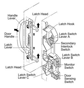
Figure D-1. Door Open Mechanism.
