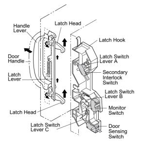
Figure C-5. Latch Switch Adjustments
