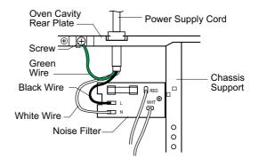
Figure C-3a. Power Supply Cord Replacement
