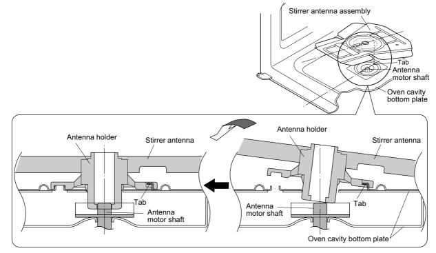
Figure C-10. Stirrer Antenna Assembly Installation
