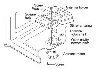
Figure C-8. Antenna Motor Shaft Removal
