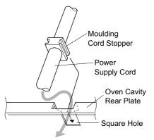
Figure C-3b. Power Supply Cord Replacement
