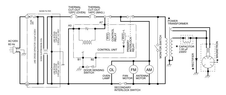
Figure O-2. Oven Schematic-Cooking Condition
