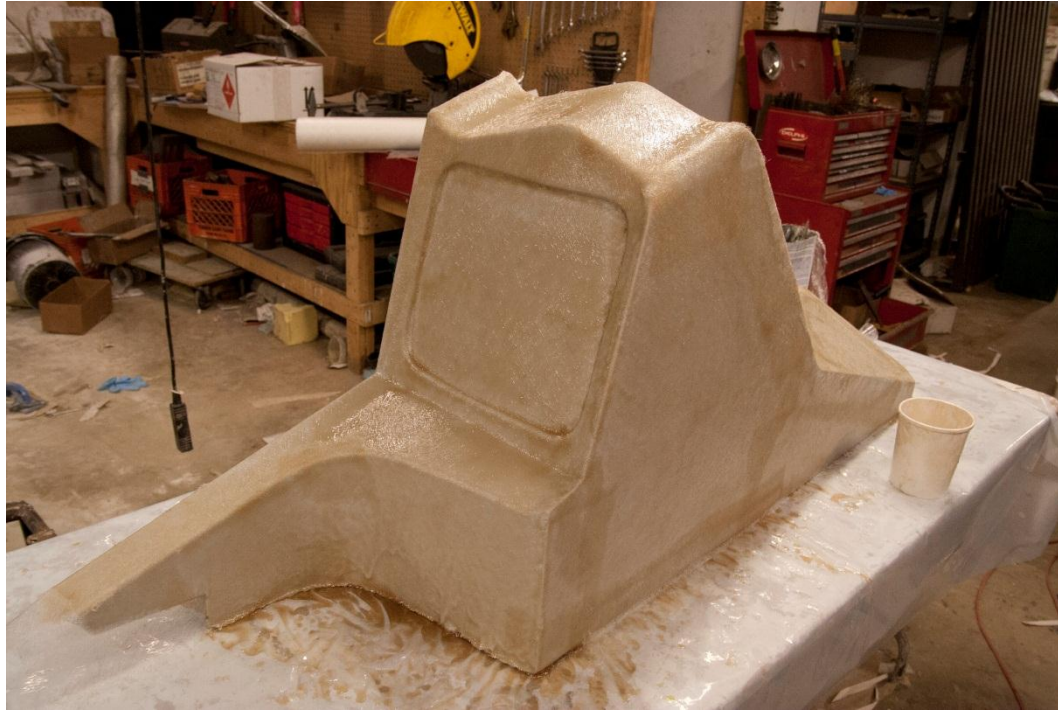
Skim coat of fiberglass
