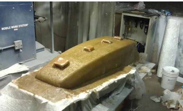
Top side fiberglass mold
