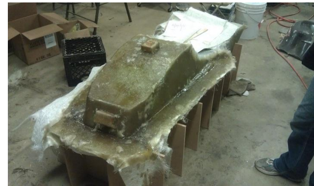
Bottom side fiberglass mold
