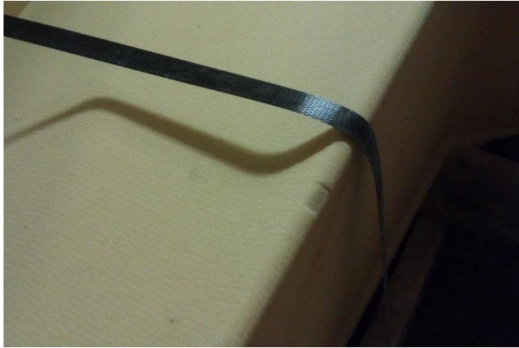
Damage due to slipped edge-guard
