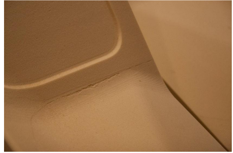
Crumbling foam joint made preCNC
