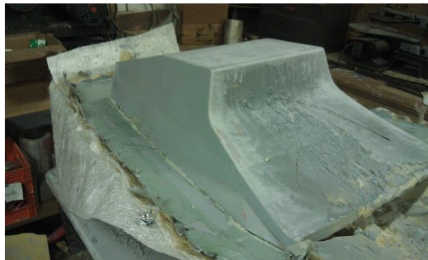
Bottom side after flange removal
