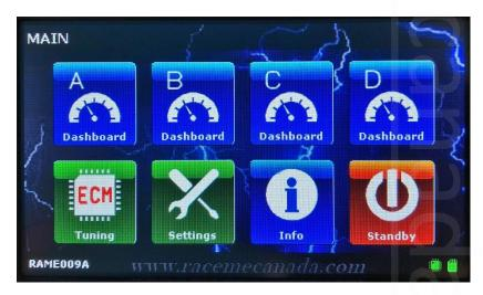
Once the tuner is up to date, turn the key to the run position without starting the truck. If you have a push button, push the button twice without touching the brake. If connected properly, the tuner will power itself on. Once you agree to the disclaimer, the tuner will default to dashboard A (gauge display).
