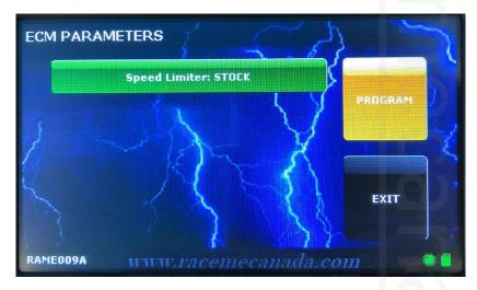
To change this value, touch the green speed limiter bar and then type in the desired value (25MPH – 250MPH) and push enter.
