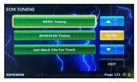
The "Get Stock file for Truck" option is only used when custom tuning is desired. This function only creates a stock file image to the SD that can be emailed to a custom tuner.
