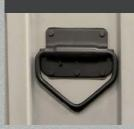
Lift / Tie Down Rings Hoisting and tie down attachment points, 2" (50 mm) diameter clearance for hooks, spring loaded, pivots 180 degrees. Plated Steel and Stainless Steel (1000lb/ring rating).
