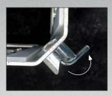
Rack is unlocked for rack removal
