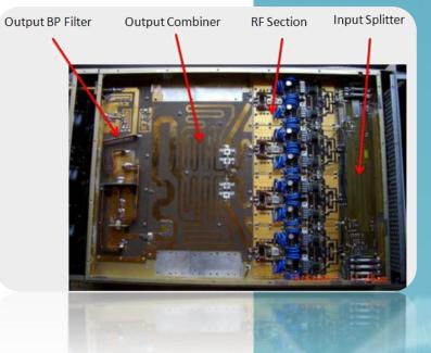
This open-cover picture shows a detailed (upper side) view of a 5kW transmitter model RAD-5 (factory-nicknamed "dash 5").
