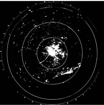
Airport Surveillance Radar S Band Detection Range - 60 nmi on a 1 m<sup>2</sup> target
