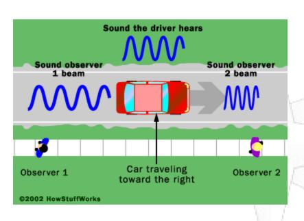
Doppler shift occurs when sound is reflected off of a moving object.
