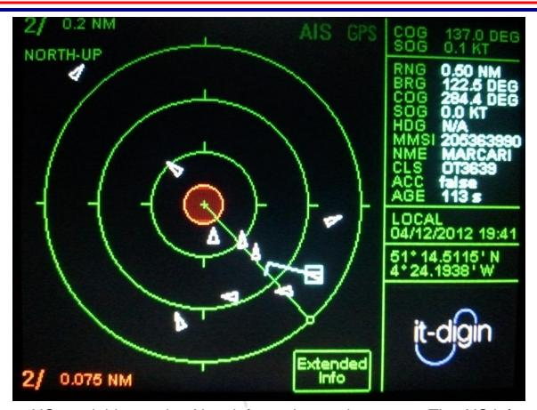
AIS overlaid on radar. Note information on the screen. The AIS info (in white) is displayed for the target with the box around it.
