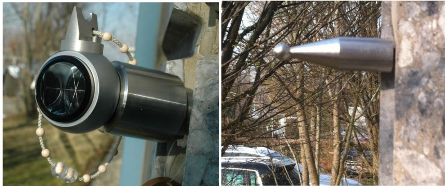
Figure 14. Constrained centring magnetic spherical prism and pin point target
