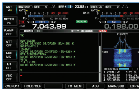
PHOTO 5: IC-7851 RTTY decoder display.
