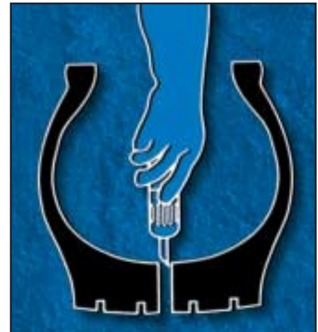
Figure 10.6 Brush chemical cure cement on nozzle and insert into the hole while turning clockwise.
