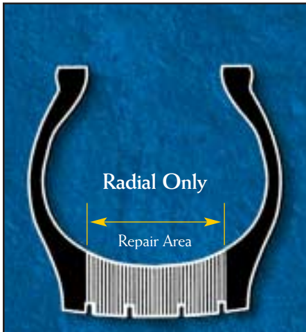
Figure 10.2 Any number of repairs in the approved crown area only tread minus outer 1" area (use outer grooves as a guide). Refer larger injuries to a full service repair shop. Do not overlap patches.
