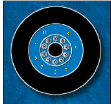
Figure 3.8 Proper sequence for tightening stud nuts on 10 stud system.
