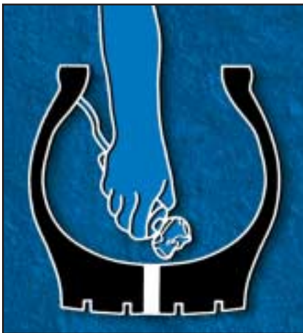
Figure 10.9 If necessary, repeat the liner cleaning procedure with pre-buff cleaner. Using a low-speed grinder, buff the liner to an RMA1 texture finish. Then vacuum to remove dust and debris.
