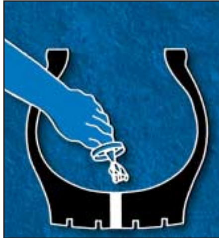
Figure 10.10 If using a chemical cure repair patch, cement the back of the patch and the buffed liner with chemical vulcanizing cement. If using a "Versacure" type repair patch, cement the buffed liner only. Thoroughly cover the cemented areas with a light, even coat. Allow proper drying time before applying the repair patch.
