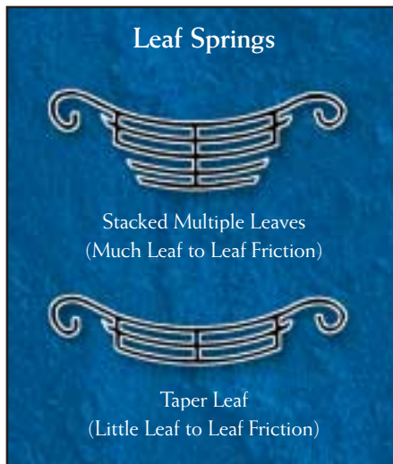
Figure 7.5 Taper-Leaf springs produce little self-damping.
