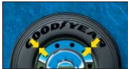
Figure 3.4 Use of GG ring to indicate correct mounting
