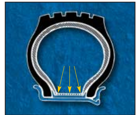
Figure 3.2 Area of tube stretched thin due to improper lubrication and mounting.
