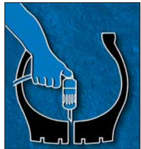
Figure 10.7 Apply air pressure (80 psi) to top of gun. This presses the plug through the nozzle into and through the injury. Remove the gun while turning in a clockwise direction.
