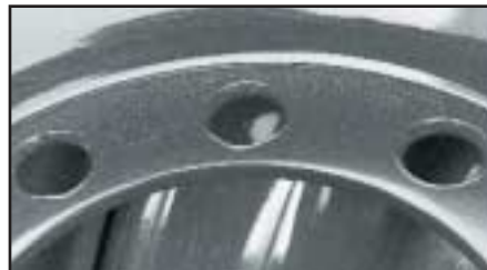
Mating surfaces should be clean, smooth, and flush so as to permit uniform distribution of clamping and torquing forces.
