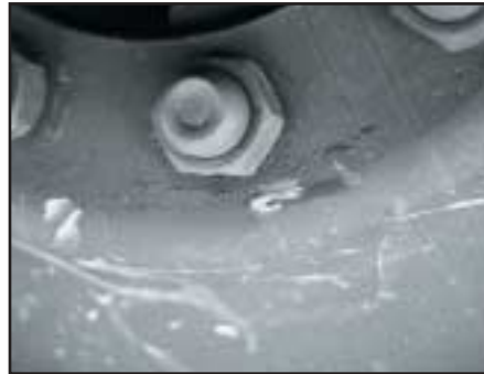
Inspect wheel mating surfaces for chaffing, corrosion or pitting.
