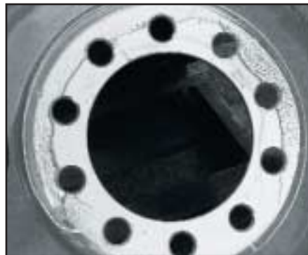
Inspect wheel mating surfaces for chaffing, corrosion or pitting.
