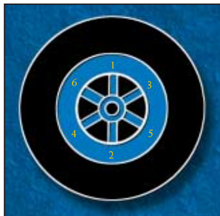
Figure 3.7 Proper sequence for tightening stud nuts on an 5 and 6 stud systems.
