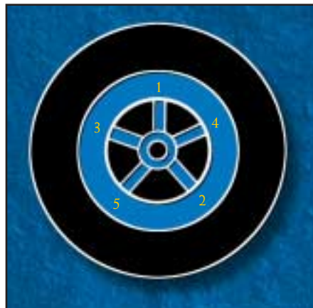
Figure 3.7 Proper sequence for tightening stud nuts on an 5 and 6 stud systems.
