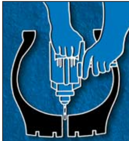
Figure 10.4 Beads in relaxed position. Using a carbide cutter, drill the injury from the inside to clean and prepare the injury for the plug.
