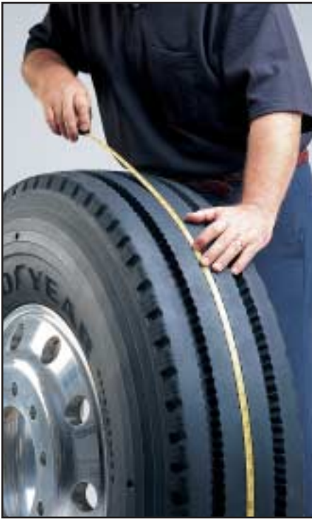
Figure 3.5 Measuring with pocket size steel tape.
