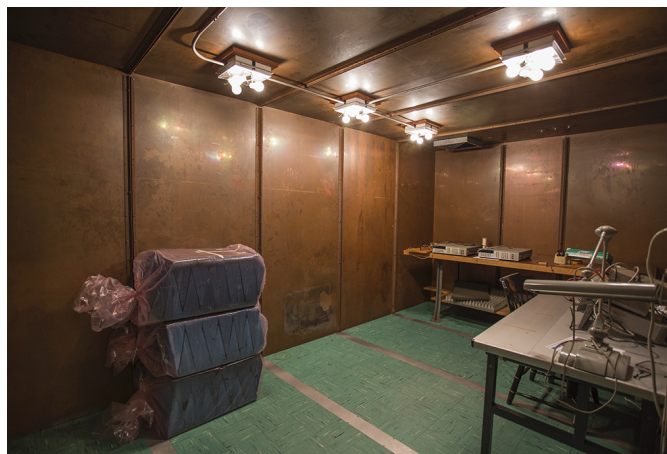
Figure 3. Zero Gauss chamber at the Climate and Space Research Building.
