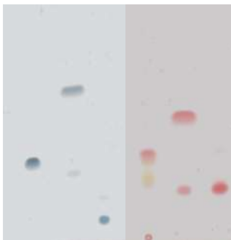
Fig. 2. Paper chromatography for remazol black (a) and for remazol orange 3R (b): migrations from left to right indication hidroxí; to sulphate; to vinyl forms.
