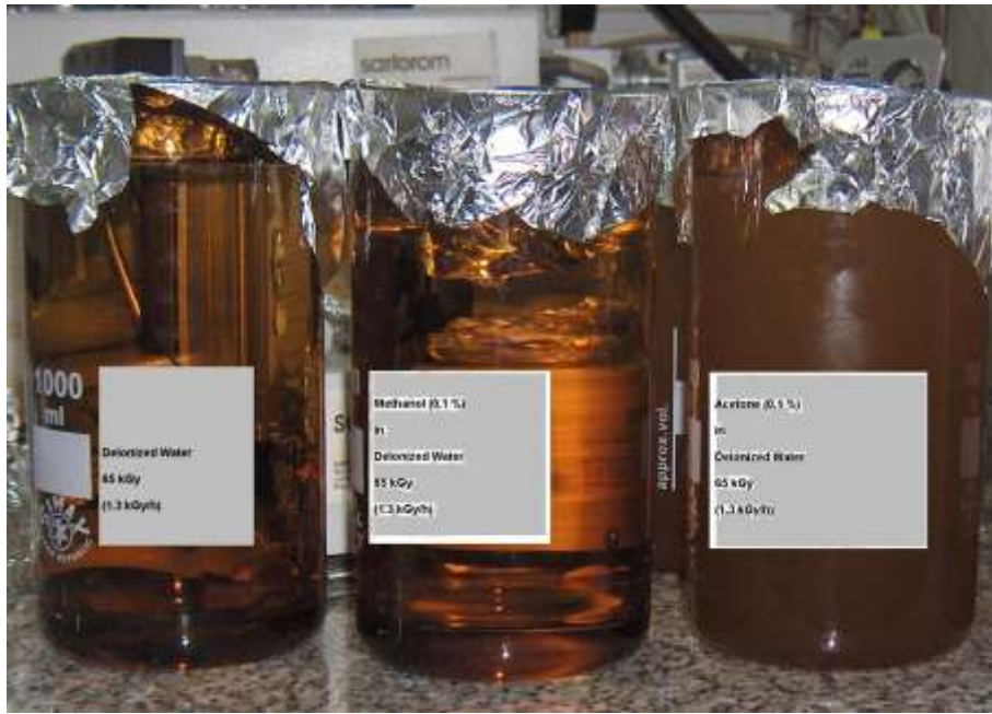
Fig. 2. First irradiation experiment for establishing the chemical stability of spiking solvents when subjected to irradiation treatment.
