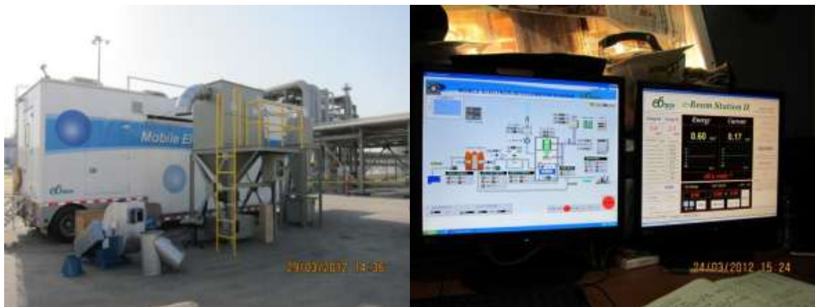
Fig. 4. Mobile Electron Beam Plant (MEB) in flue gas treatment in Jeddah, Saudi Arabia.
