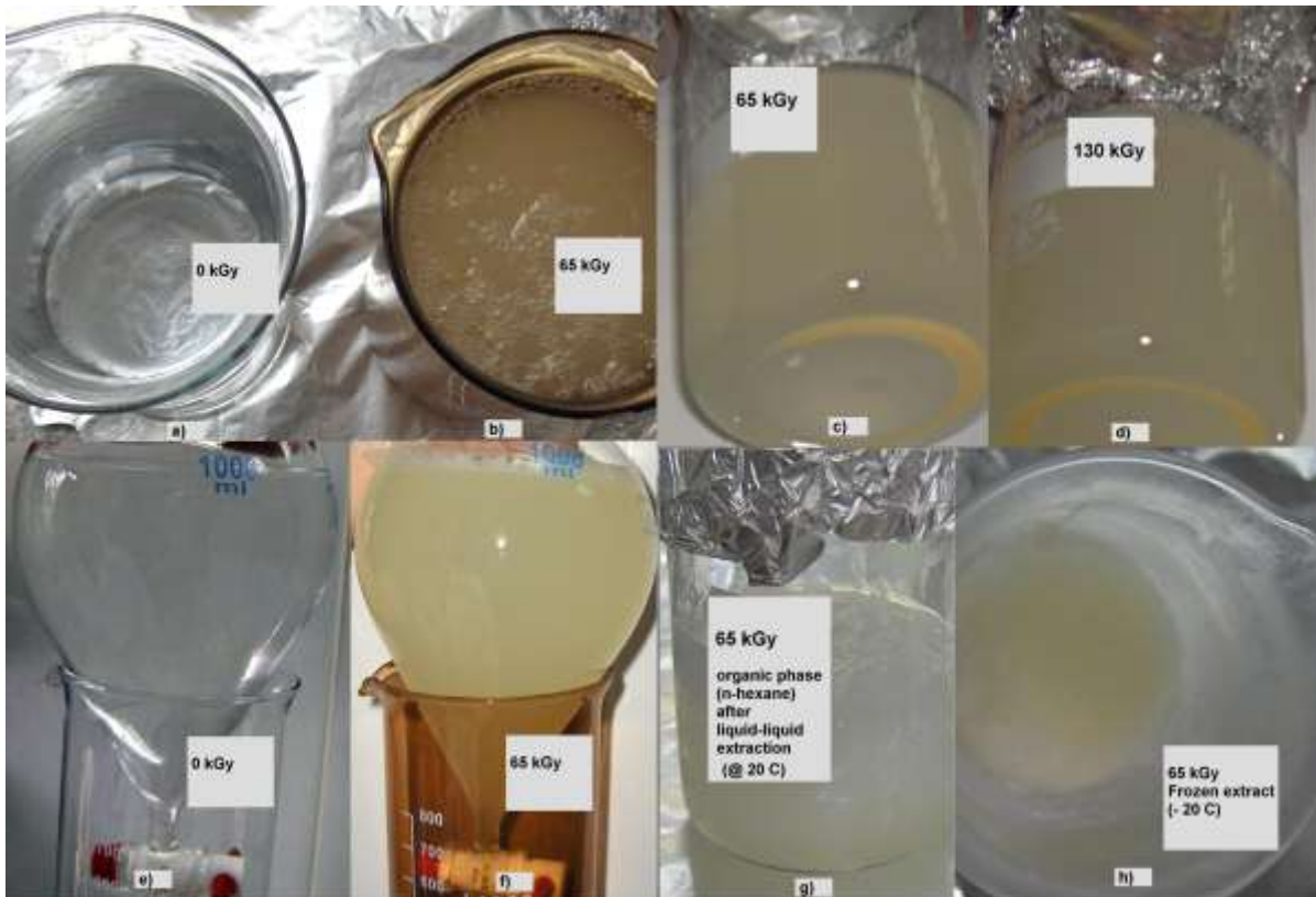
Fig. 1. The initial irradiation experiment of acetone (0.1% in deionised water) as spiking solvent for PCB 52 and HCB (having a concentration of 1 ppb in deionised water, obtained by adding 1 ml of acetone with 1 ppm of POPs to 1 l of deionised water): a) - f) unirradiated & irradiated positive quality controls before and after liquid-liquid extraction; g) & h) organic phase collected after liquid-liquid extraction before and after separation from interfering matrix by freezing at -20\text{ }^{\circ}\text{C} .
