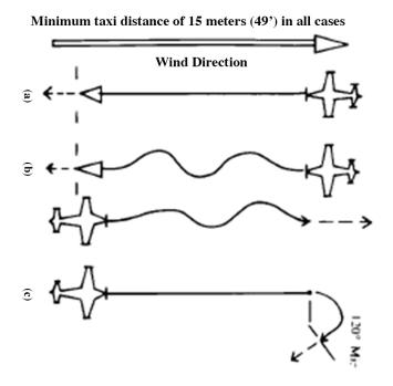
a. Models with two-wheel landing gear and tail skid or unsteerable tail wheel, or other gear configurations not allowing steering will taxi forward into the wind a distance of at least 50 feet, slow down to a near stop or stop, and then become airborne in a realistic manner.
