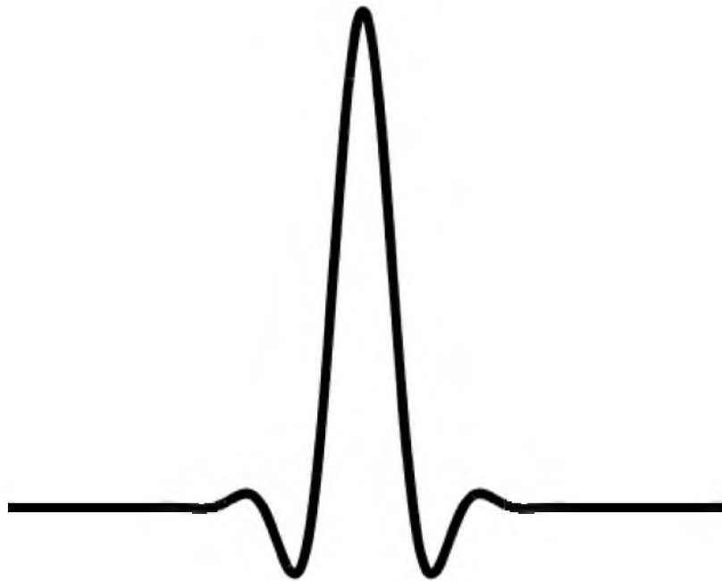
Figure 1.2. The finite bandwidth pulse used in an 802.11b channel sounder.
