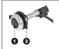
Both shafts are designed for a front and rear knob plus push functionality. The illustration on the left shows the left shaft (labeled 1 and 2 in Figure 10) with knobs installed. Use the Operation table to determine how to use the knobs to achieve the desired response from your "Model Hermosa" radio.
