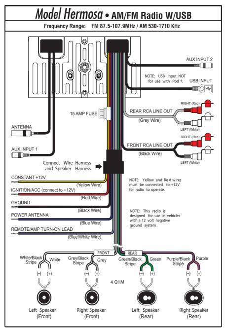
Figure 9 - Wiring Diagram
