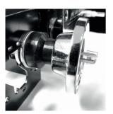
Figure 5 - Shaft Cover Installed
