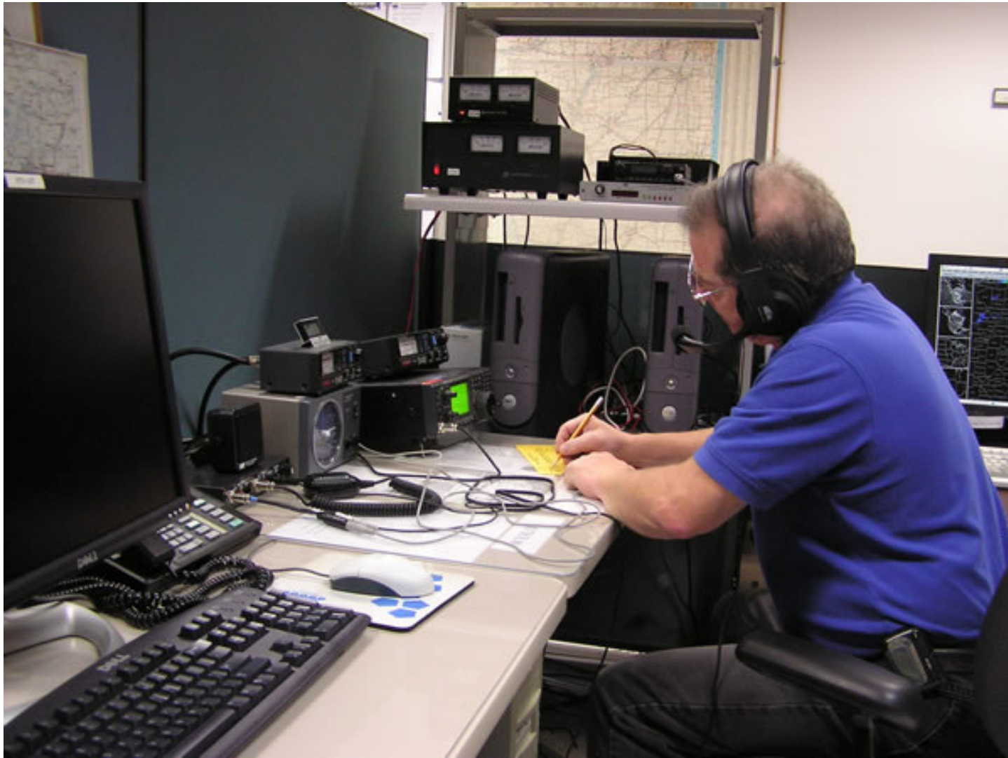
A Typical Modern HAM Shack With Radios, Power Supplies, And the Ubiquitous Computer/s
