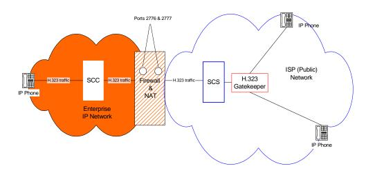
*Figure 4-1* illustrates a typical configuration using the Secure Communicator.
