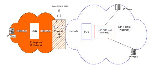
Figure 4-2 Secure Communicator and viaIP
