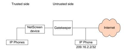
Figure 2-5 Untrusted Gatekeeper (Transparent or Routed Mode)
