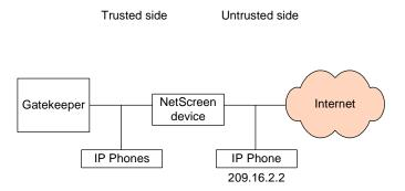
Figure 2-3 Trusted Gatekeeper (Transparent or Routed Mode)
