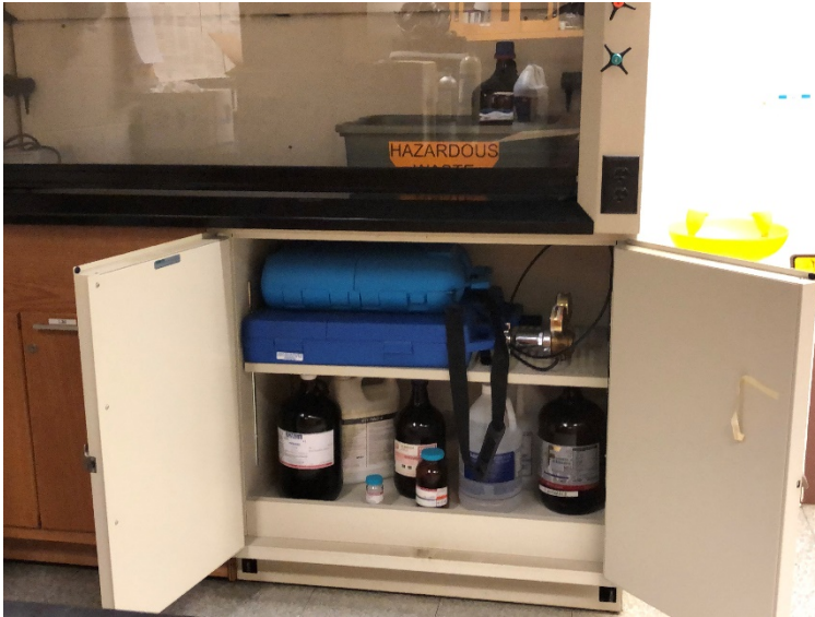
Cylinder protective cases on shelving under fume hood
