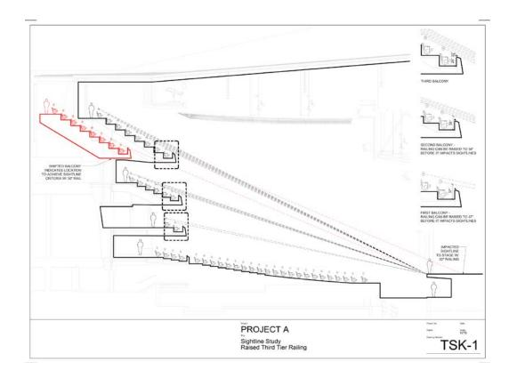
Figure 2. Red lines show the effect of raising the railing in the upper balcony area (Rosenbaum, 2019)
