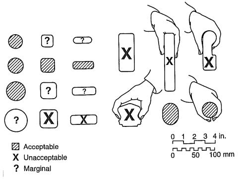
Figure 6. Cross Sections of Railings (NFPA, 2009).
