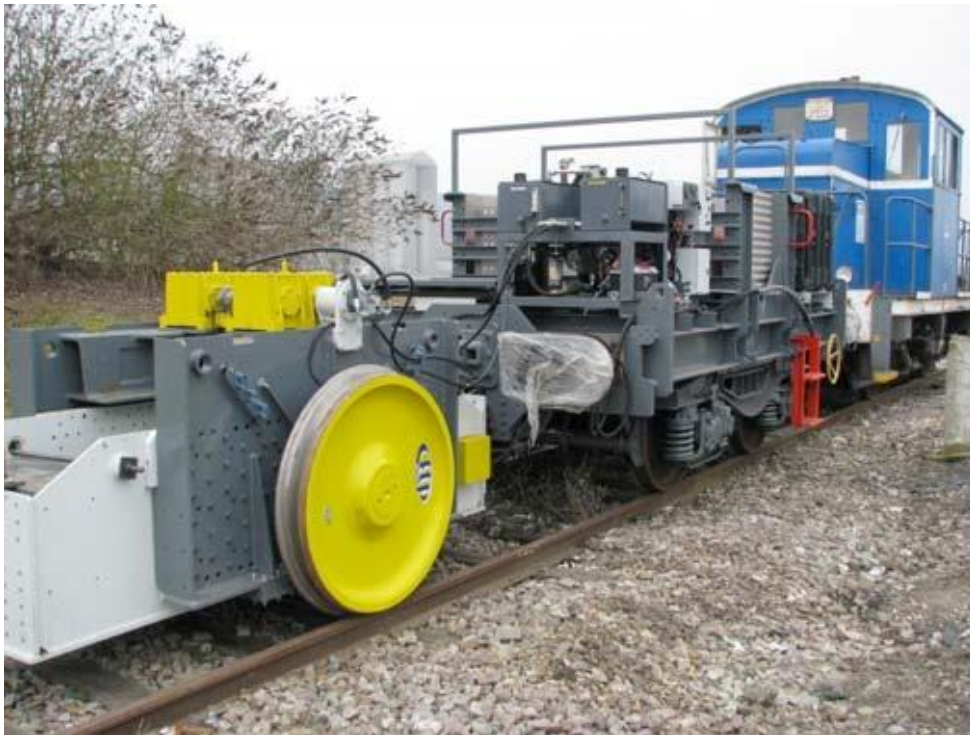
Figure 23: A version of the adapted Portancemètre during its development (LCPC and CETE, 2007)
