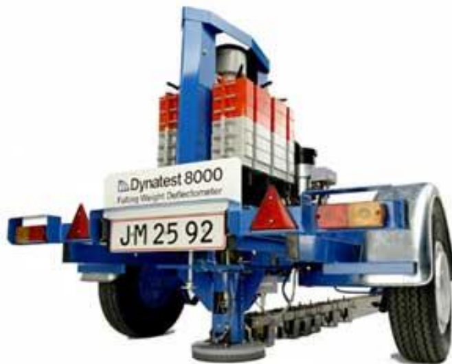
Figure 19: Typical FWD mounted on a trailer for use on highway pavement surfaces. (Dynatest)
