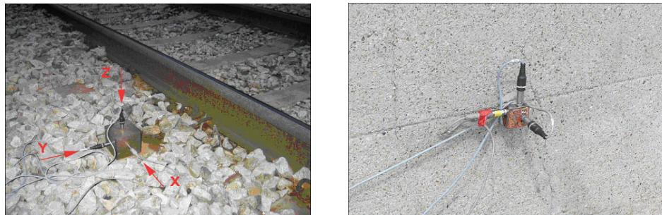
Fig. 5 Measuring devices for vibrations
